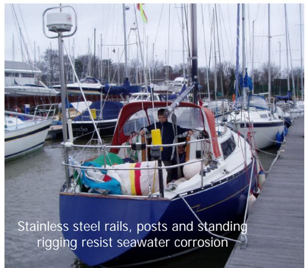
Stainless steel rails, posts and standing rigging resist seawater corrosion
